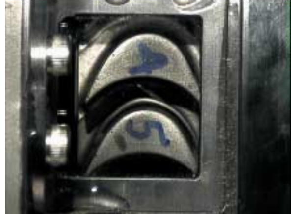
Figure 7 A view of the rotor blades through the laser velocimeter optical window
