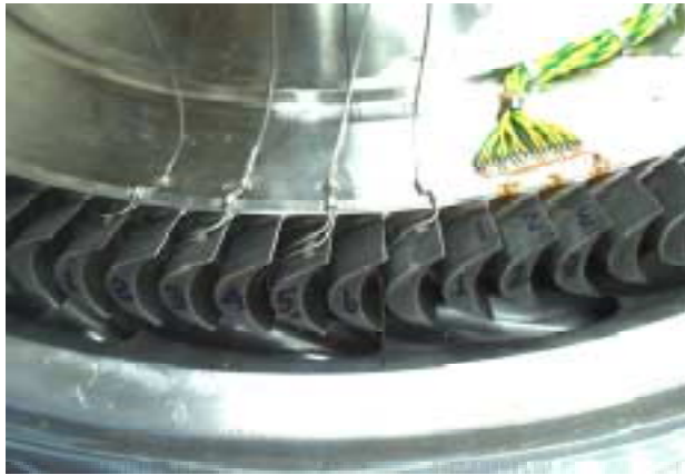
Figure 6 Instrumented rotor blades for wall static pressure and strain gage measurements
