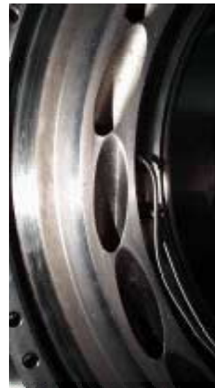
Figure 3 A view showing 3 of the supersonic nozzles
