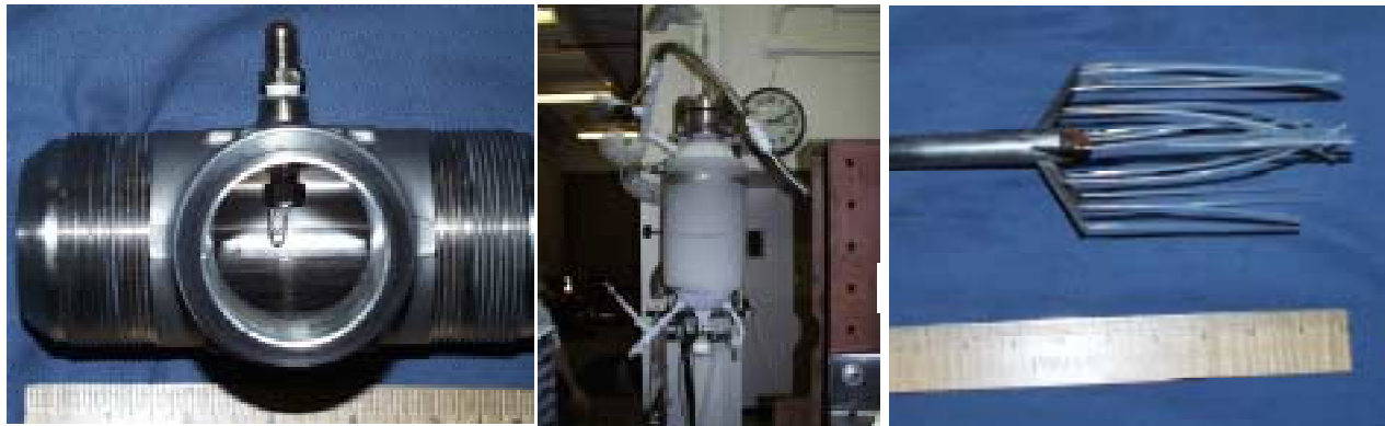
Figure 8 Atomizer in the flow pipe Figure 9 Pressurized \text{LN}_2 seeder system Figure 10 Bubbler rake used to keep \text{TiO}_2 in suspension
